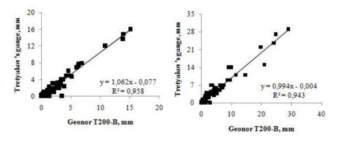
a)  $0.5 \text{ m s}^{-1}$  b)  $6-10 \text{ m s}^{-1}$ **Fig. 2.** Linear regression analysis for Tretyakov gauge adjustment to GEONOR T200-B for different wind speed ranges.
