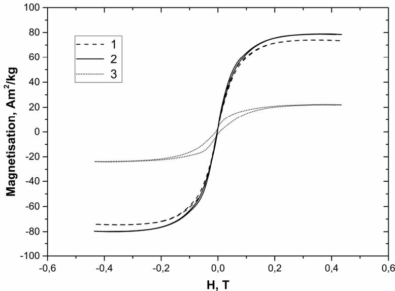
**Fig. 4.** Hysteresis loops for magnetic fraction of granodiorite (1), metagabbro (2), and microgabbro (3).
