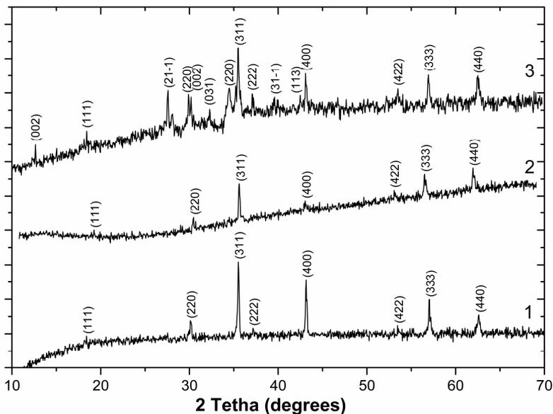
**Fig. 5.** XRD patterns of magnetic fraction of granodiorite (1), metagabbro (2), and microgabbro (3). Numbers correspond to Miller's indexes.
