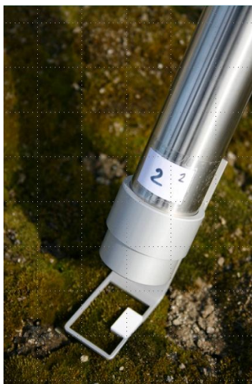
Fig. 1. View on a fluorometer head installed in the field at the long-term research plot (LTRP). The metallic frame with reflexive white plate (for PAR measurement) delimits measuring spot on Bryum sp. cushion.
