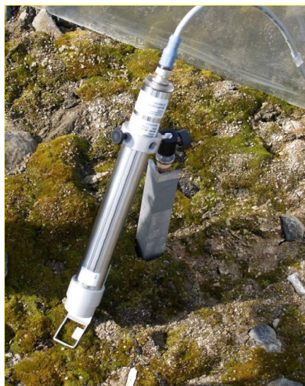
Fig. 1. View on a fluorometer head installed in the field at the long-term research plot (LTRP). The metallic frame with reflexive white plate (for PAR measurement) delimits measuring spot on Bryum sp. cushion.
