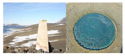
Fig. 3. Example of British stabilised points (Nr. 4001).
