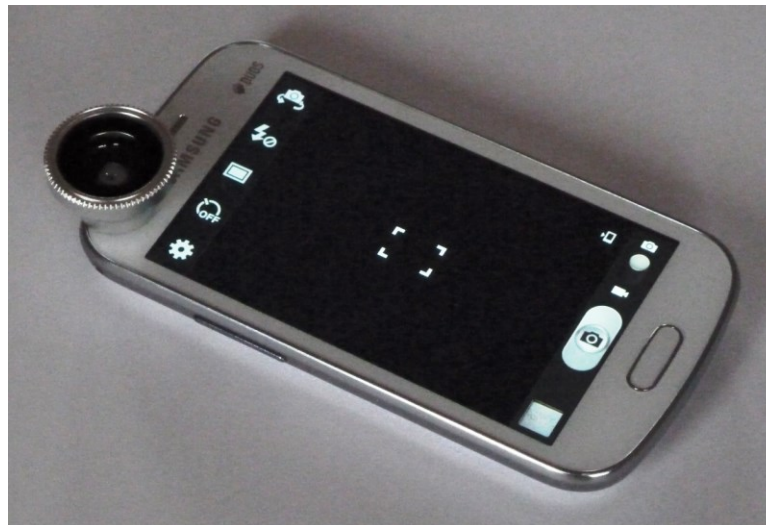
Fig. 3: External, inexpensive fisheye lens for smartphone.
