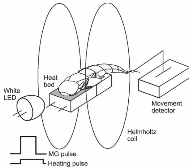
**Fig. 2.** Overall layout of the experiment. The pupa was fixed by glueing its ventral side to the heat bed. The abdominal contractions were transmitted to the movement detector and recorded on a personal computer. In conditioning experiments, a magnetic pulse (10 s) was applied together with a heating pulse (15 s). The temperature peaked at the moment of switching the heat pulse off.
