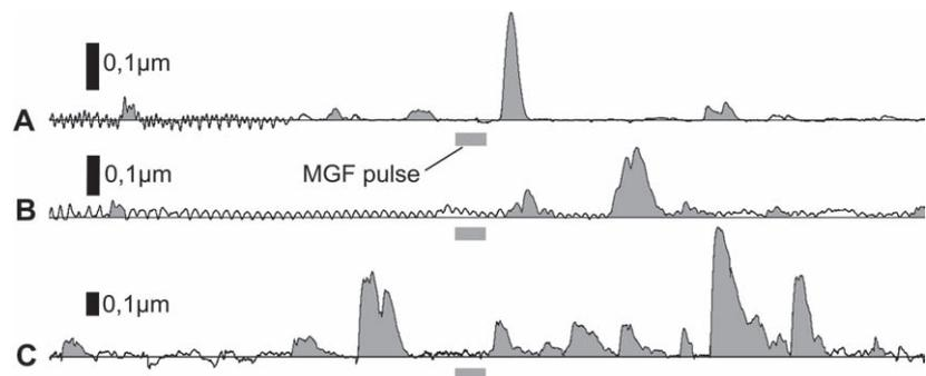
**Fig. 5.** Three examples of the test (A–C). Only a magnetic impulse without a heat shock is applied. The effective amplitudes of peaks (the grey-filled areas) were considered in the statistical evaluation. Only peaks larger than 10% of the highest peak were selected.
