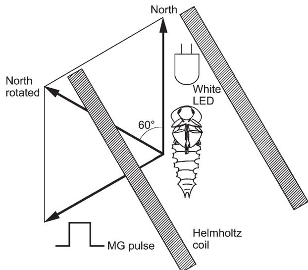
**Fig. 1.** Position of pupa and Helmholtz coil towards the geomagnetic field. The rectangular pulse lasting for 10 s shifted the north position by  $60^\circ$ . The illumination was provided by the light-emitting diode.
