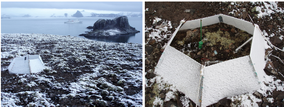
Fig. 2. Experimental site with OTCs on La Cruz Plateau after snow fall (left). Detailed view on the OTC taken immediately after a snowfall (right). Note that majority of freshly deposited snow is over the ground outside OTC while inside the OTC there is hardly any snow. Photo © M. Barták.
