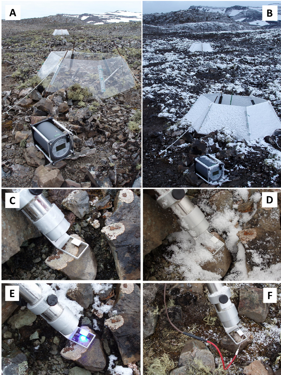
Fig. 1. Experimental set up of the MONI-PAM with measuring probes installed over Placopsis antarctica thalli. A - general view on the OTCs located on La Cruz Plateau, B - the same site after snowfall, C, D - detail of the measuring probe on the control plot (C - after a rainfall, D - after a snowfall), E - location of saturation pulse spot on P. antarctica thallus, F - detail of the measuring probe and Cu-Co thermocouple measuring air temperature at the measuring spot inside OTC. Photo © M. Barták.
