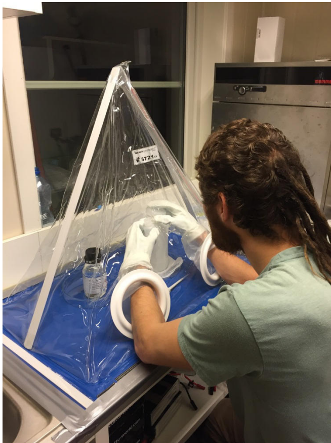
Processing the samples of snow for heavy metal analyses (photo Kristián Brat)
